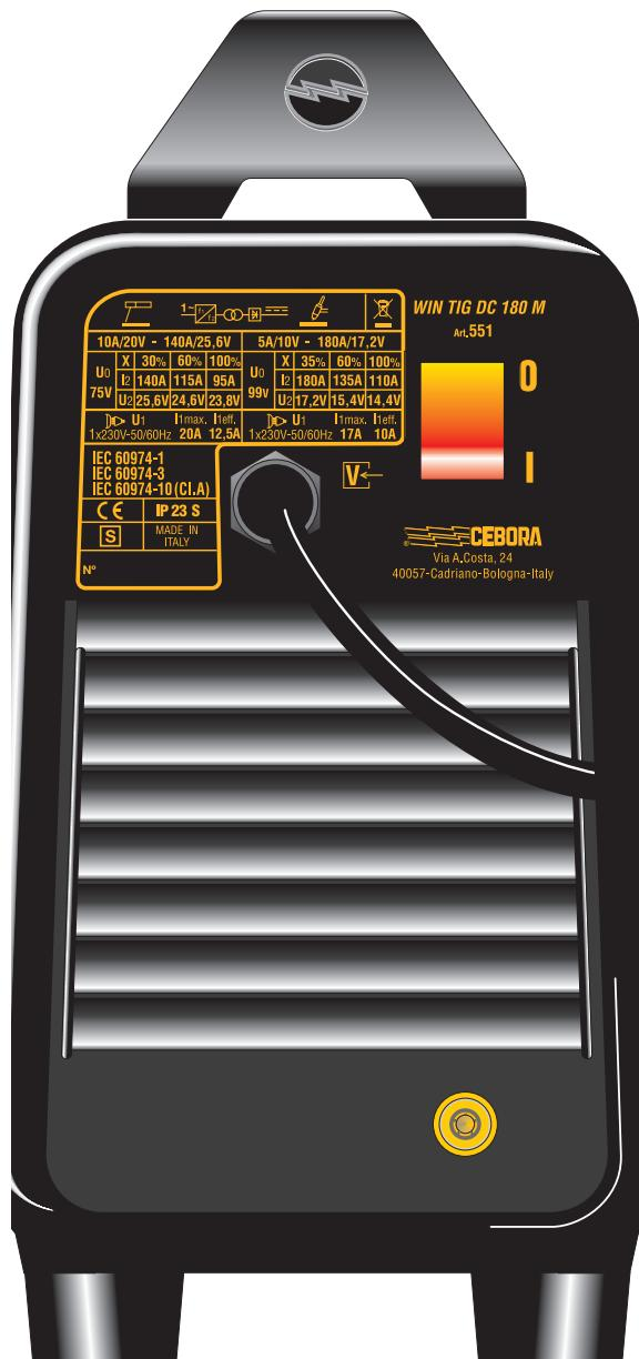
**WIN TIG DC 180 M (art. 551)** is a single-phase inverter power source (**180 A 35%**), suitable for TIG and MMA/SMAW welding, with the exception of AWS6010 cellulosic electrodes; mainly designed on purpose for maintenance and repair works, as well as small production batches.
